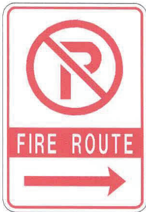
F.R. 2 Indicates direction of prohibited parking. Defines the end zones of a fire route.
